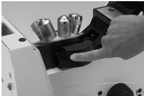
Fig. 111 DIC disk with knurled wheel for fine adjustment
