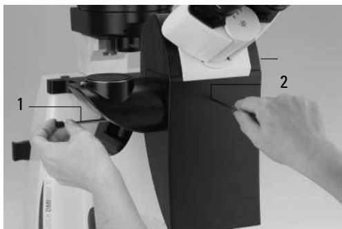
Fig. 95 Phase contrast centering procedure
