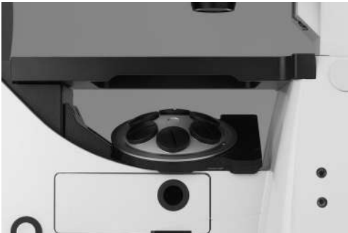
Fig. 45a Objective turret
