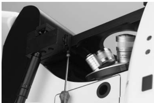
Fig. 24 Installation of attachable mechanical stage
