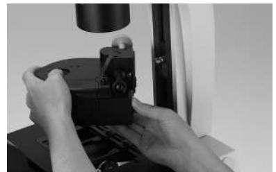
Fig. 40 Installation of condenser on transmitted light illumination arm
