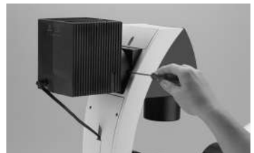
Fig. 49 Connecting the lamp housing to the Leica electronics box, example: Leica CTR6000
