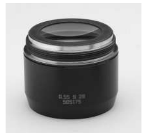
Fig. 35 Condenser head S28
