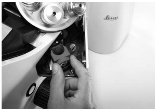
Fig. 67 Inserting or removing a filter cube
