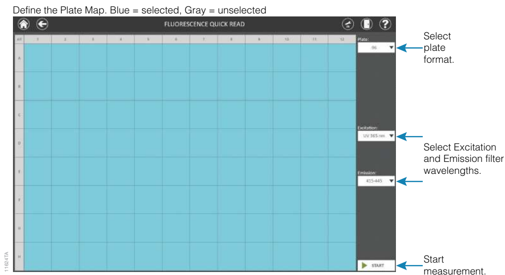
Figure 10. GloMax® Explorer ‘Fluorescence Quick Read’ screen. On the plate map, blue wells are selected.
