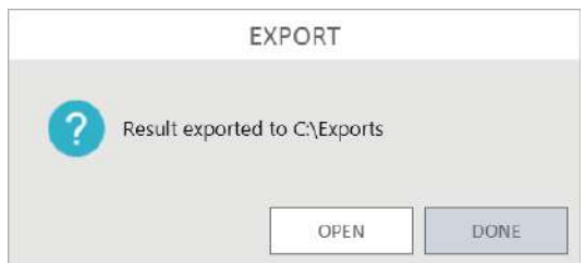
Figure 58. Export of results. This screen is displayed upon the successful export of results to the administrator-defined manual export location. Use the Open button to open the export location in a Windows ® file browser or tap the Done button to return to the results plate map.
